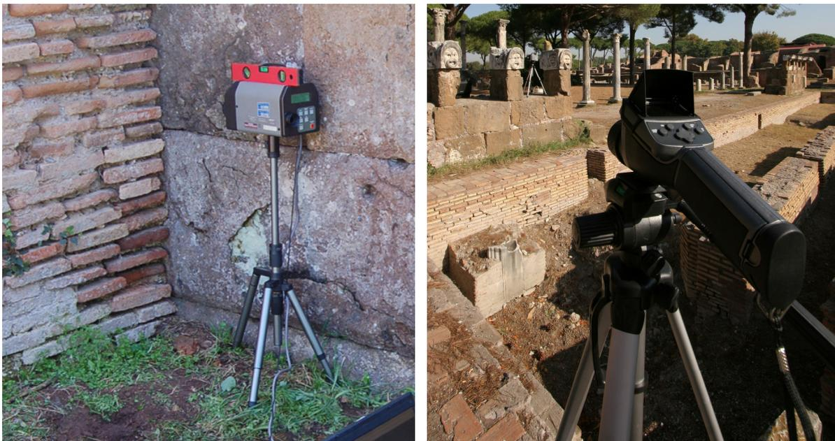
Figure 4: The spectroradiometer Minolta CS-1000A (left).
